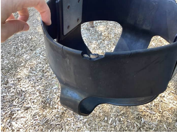
Sharp point at swing
