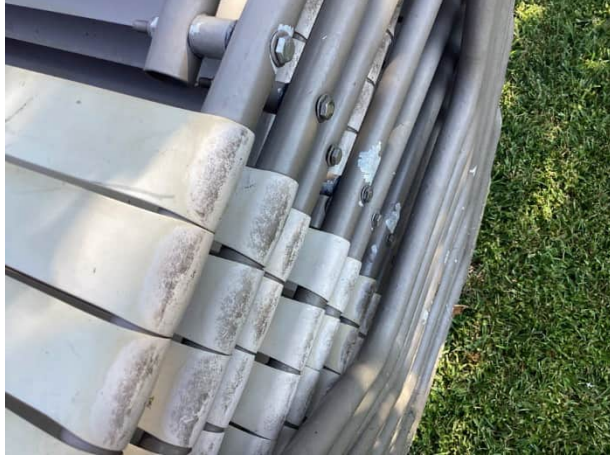
Frame finish deterioration
